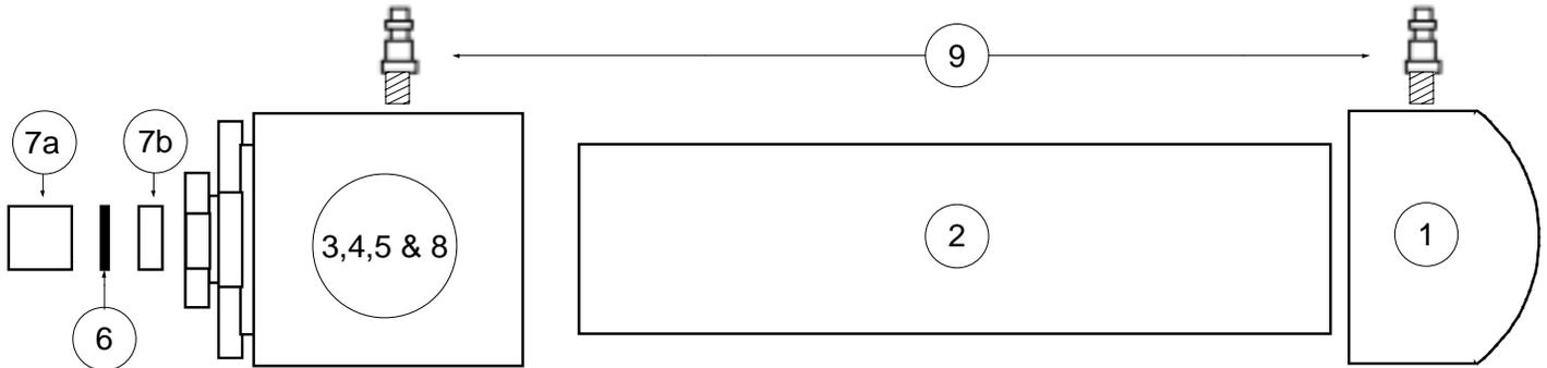
Use PVC cement and clamp all assemblies together, for a tight fit. All fixtures need at least 6 hours to cure before the clamps are removed.
